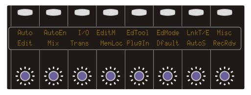
The two soft key sets are called **User 1** and **User 2**, and are activated by pressing the **User 1** or **User 2** switch, below the Nucleus logo in the centre section. The top row of the scribble strip display indicates the Mode switch function, the bottom row the V-Sel function. To return the Mode and V-Sel switches to their normal functions, deselect both **User 1** or **User 2** switches.
